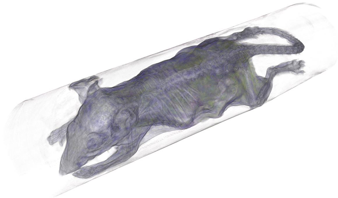
Fig. 5 3D visualisation of the plastimouse CT reconstruction. The data were measured using the RadalyX robotic scanner.
