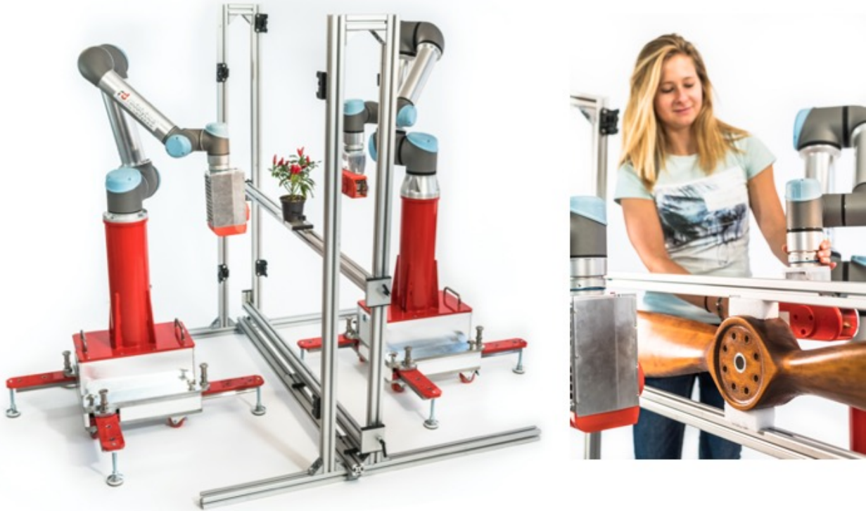
Fig. 1 Photography of the existing robotic scanner RadalyX for general inspection applications. The device allows large area 2D scans, computed-tomography and real-time X-ray inspection.
