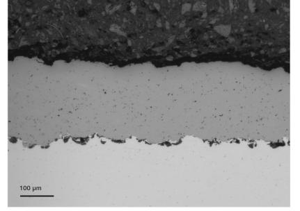
Cold-sprayed tantalum coating on 316 stainless steel. Sample provided by TWI Ltd
