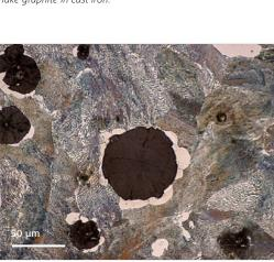
Spheroidal graphite in cast iron, taken in brightfield mode. Images provided by University of Applied Sciences, Aalen, Germany
