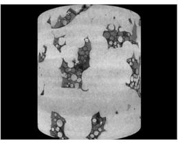
3D printed part from powder steel: Solid domain. Sample courtesy of NIST
