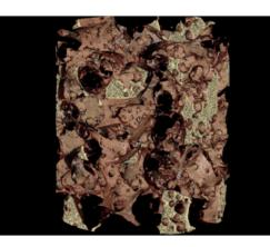
3D printed part from powder steel: Pore domain. Sample courtesy of NIST
