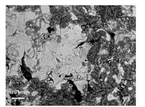
Surface of corroded mild steel.
