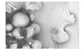
Surface of additively manufactered titanium alloy component. Sample provided by TWI Ltd
