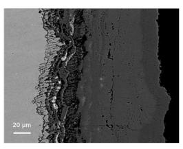
Corrosion scale formed during high temperature oxidation of 9% Cr steel. Sample provided by TWI Ltd
