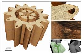
3D scan of Al component produced by additive manufacturing and, inset, internal porosity imaged via X-ray microscopy
