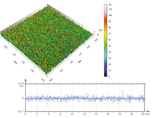
Height map and example line profile of grit blasted metal surface. Sample provided by TWI Ltd.
