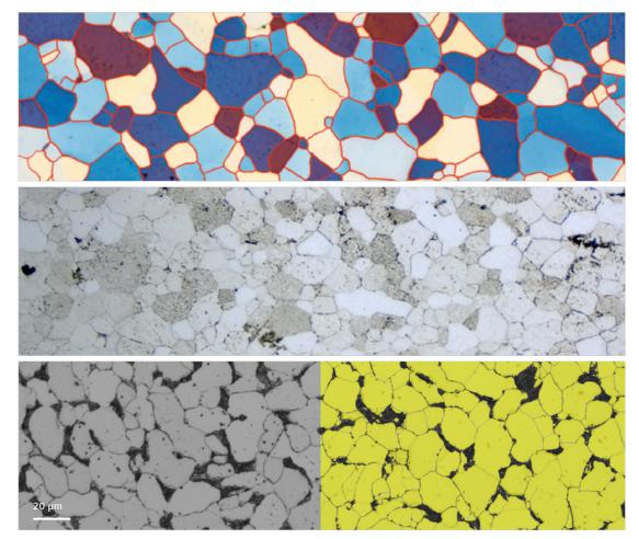
Measurements of grain size in ferritic steels
