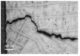
Cracking in nickel Alloy 825 casting. Sample provided by TWI Ltd
