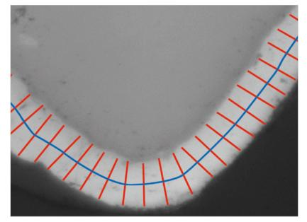
Layer thickness measurement on curved surface.
