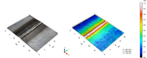
3D scans of root of autogenous nickel alloy weld using ZEISS Smartzoom 5 tilting and height rendering functions. Sample provided by Haynes International, Ltd
