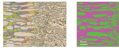
Measurement of ferrite content in the vicinity of a weld in duplex stainless steel. Sample provided by TWI Ltd
