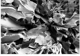
Steel fracture face after failure in tension. Sample provided by The Test House, Cambridge
