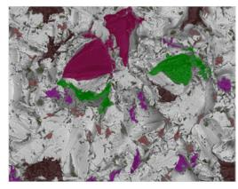
EDS map depicting categorized alumina particles on surface of \$355 structural steel after grit blasting with F80 grit. Sample provided by TWI Ltd UK
