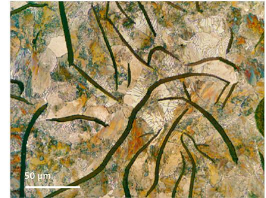
Flake graphite in cast iron, etched sample
