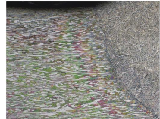
Parent to weld interface in duplex stainless steel. Sample provided by TWI Ltd
